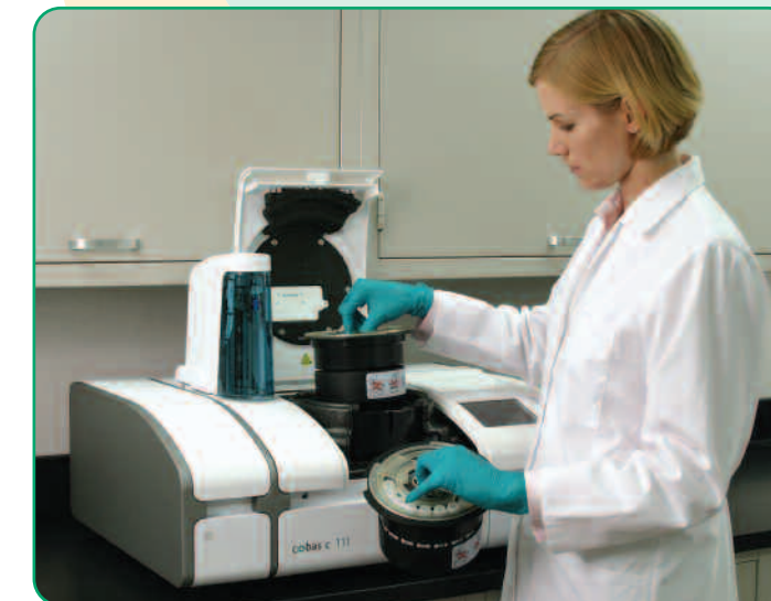
Cooled, exchangeable reagent disc
